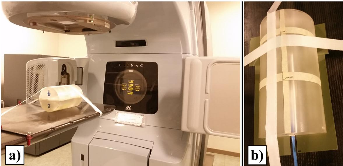
Figure 2.22: a) Photo of the experimental setup, the 14-cm diameter PMMA cylindrical phantom is on the patient bed stopped with scotch tape (first plane) and the Clinac irradiate a cylindrical volume with the beam size of  $1.5 \times 2.0 \text{ cm}^2$  (background). b) 14-cm diameter PMMA cylindrical phantom with three EBT3 film inserted in the mid-plane.
