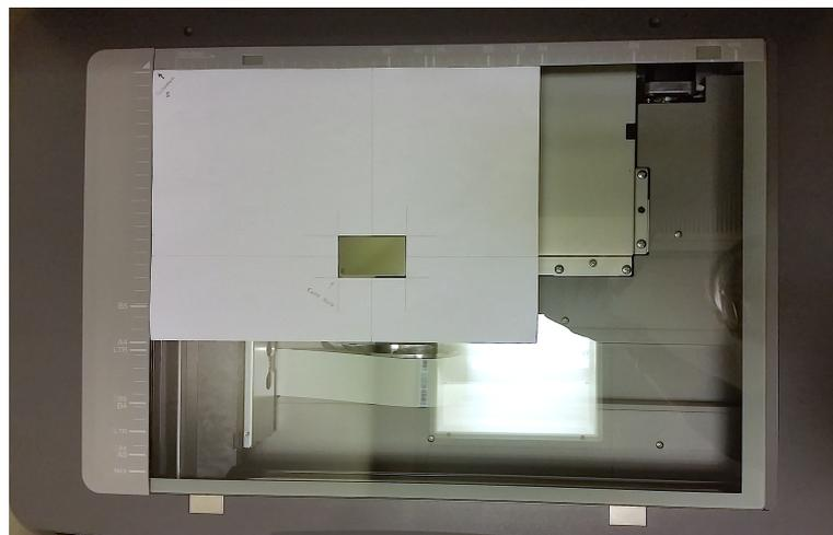
Figure 2.11: EBT3 film piece positioned in the scanner with the help of a paper guide.
