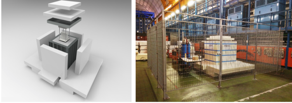
Figure 2.4: Schematic (left) and real (right) picture of the shielding for the technical test installed in underground Gran Sasso laboratory.
