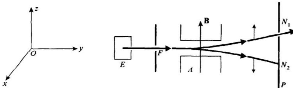
Figure 1.1: Schematic drawing of the Stern Gerlach experiment.
