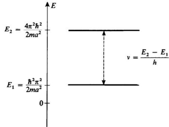
Figure 3.2: Energy spectrum in the infinite barrier approximation.
