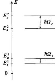
Figure 3.4: Energy spectrum in the finite barrier approximation.
