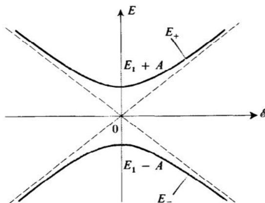
Figure 3.6: Anticrossing diagram for the Ammonia molecule in a static electric field pointing towards the axis of symmetry of the molecule.
