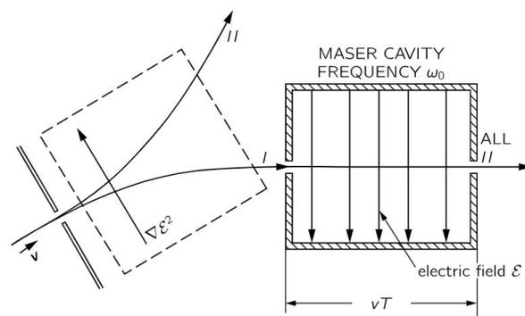
Figure 3.7: Schematic drawing of the Ammonia maser.
