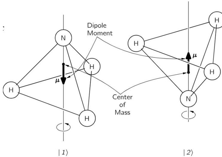
Figure 3.5: Two level system model for the Ammonia molecule in its ground state.
