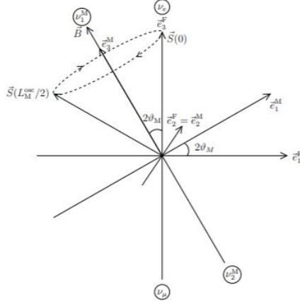
Figure 5.1: Neutrino oscillation on the Bloch sphere.
