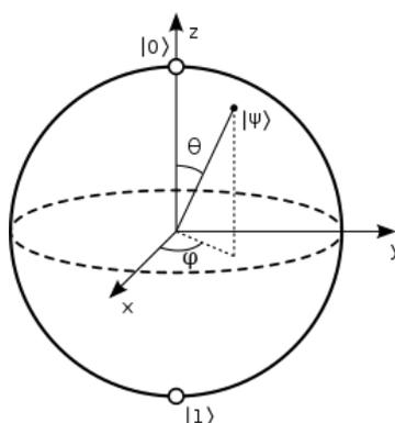
Figure 1.3: Geometrical representation on the Bloch sphere.
