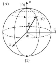
Figure 1.4: Quantum mechanical Larmor precession on the Bloch sphere.
