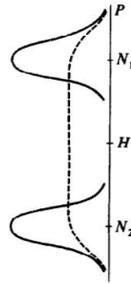
Figure 1.2: Spot observed in the Stern Gerlach screen. According to classical mechanics one should observe one spot (dashed line), in reality two symmetrical spots centered at  $N_1$  and  $N_2$  are observed.
