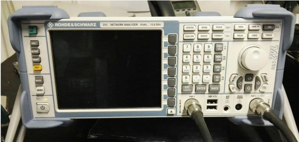
FIGURE 3.6: Front view of the Rohde&Schwarz Vector Network Analyzer ZVL6, which is a two ports VNA. The electronic connection with the device under test can be created through the ports at the bottom. The various buttons allows to set different features of the VNA, as well as changing its functioning modality. The results of the measurements are shown on the display.
