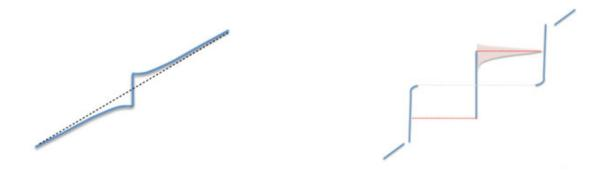
Figure 1.13: **Left**: Current-Voltage Characteristic for an over-dumped junction. **Right**: Current-Voltage Characteristic for an under-dumped junction [23].
