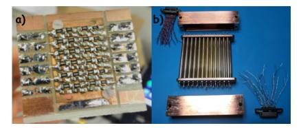
Figure 2.5: **a)** Image shows a series of RC filters used for DC lines in the Tryton system.**b)** Assembly of copper powder filters.
