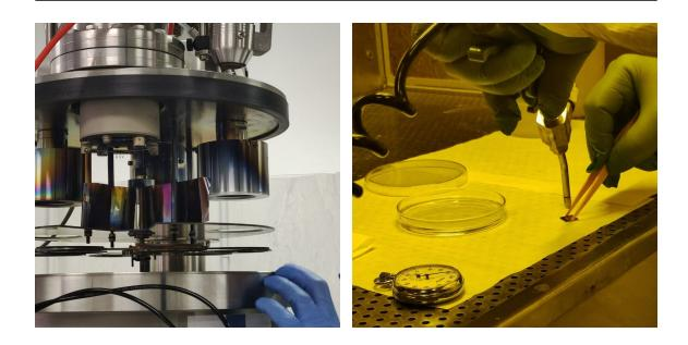
Figure 3.2: Left: Photo depicting the positioning of the chip inside one of the chambers of the rotating sputtering system at the CNR in Pozzuoli. **Right**: Chip development and cleaning after aluminum deposition.
