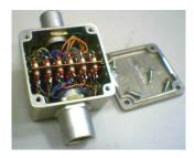
Figure 2.4: EMI filters installed on the Tryton system are shown.
