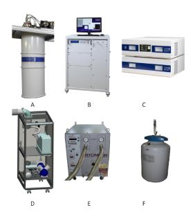
Figure 2.1: Triton consists of six stand stand-alone components: cryostat with pulse-tube cooler (A); gas handling and control rack (B); magnet power supply rack (if required) (C); pump rack (D); pulse-tube compressor (E) and a liquid nitrogen dewar with cold trap (F) [36].
