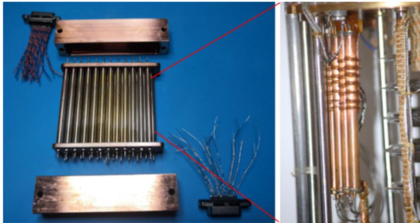
Figure 3.4: Picture of the copper powder filters, in the box on the right a detail of the internal structure of the copper cylinders.
