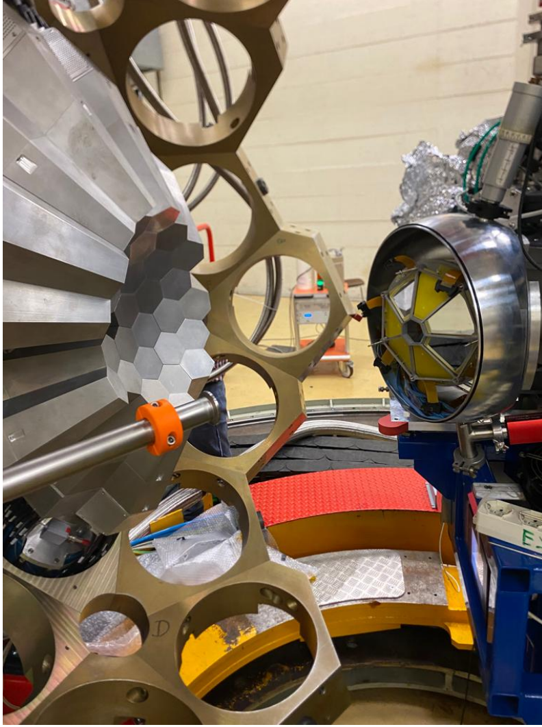
Figure 4.1: The experimental setup, composed of the AGATA and SPIDER arrays.
