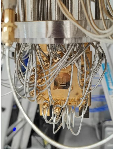
Figure 22: Contralto-D QPU stage: at the center, the copper-plated cavity which hosts the qubits; on the edges, the qubits drive and flux lines, and feedlines connections.
